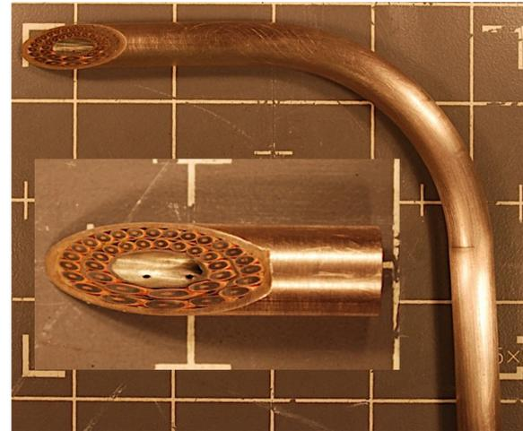
Fig. 12. Sample of 2-layer CIC, bent on 61 mm bend radius. Inset: cross-section cut on 45° bevel to show inner structure.
