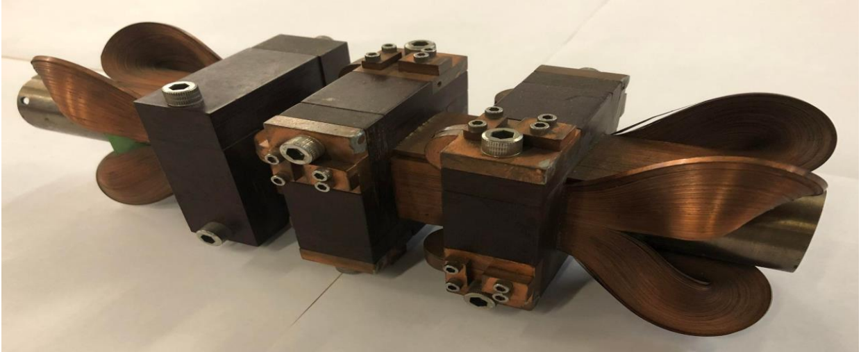
Figure 5. Example of flared ends in a tape-stack cable: Sampson's flared-end quadrupole using dip-coated \text{Nb}_3\text{Sn} superconducting tape.
