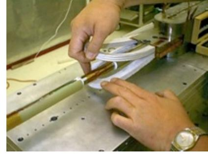
**Figure 6. Spreading the inner windings to clear the beam tube.**
