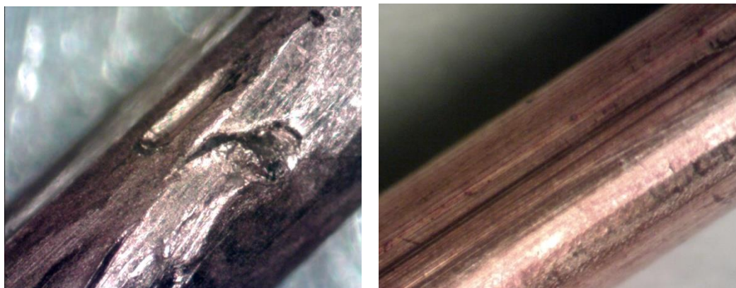
Figure 5. a) single-layer over-wrap carved divots in the wires of the inner layer; b).a multi-layer over-wrap was applied between inner and outer wire layers, there was no surface damage.
