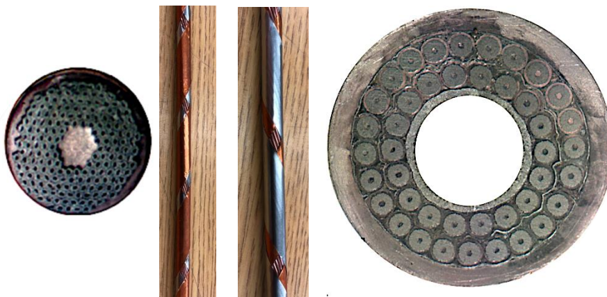
Figure 7. 2-layer \text{Nb}_3\text{Sn} SuperCIC: a) HyperTech's tube-process \text{Nb}_3\text{Sn} wire, b) over-wraps of inner layer 316SS and Cu foil tapes applied; c) outer layers of Cu foil and 316SS tapes applied; d) finished SuperCIC.
