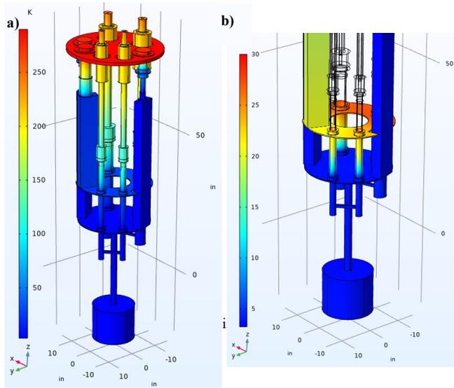
Fig. 4. Temperature profiles of a reduced model of the cryostat at the end of two stages of operation: **a)** after cooldown, with no currents active; **b)** full rated currents in all 4 leads, equilibrium after one hour (data range has been restricted for better visualization).
