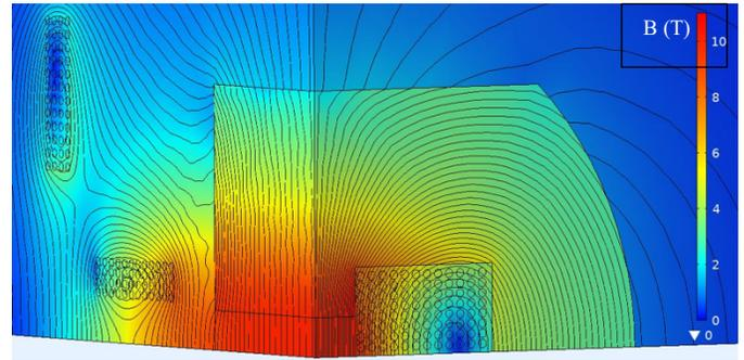
Fig. 6. Cutaway view of magnetic field distribution in one octant of the 10 T CIC background-field dipole.
