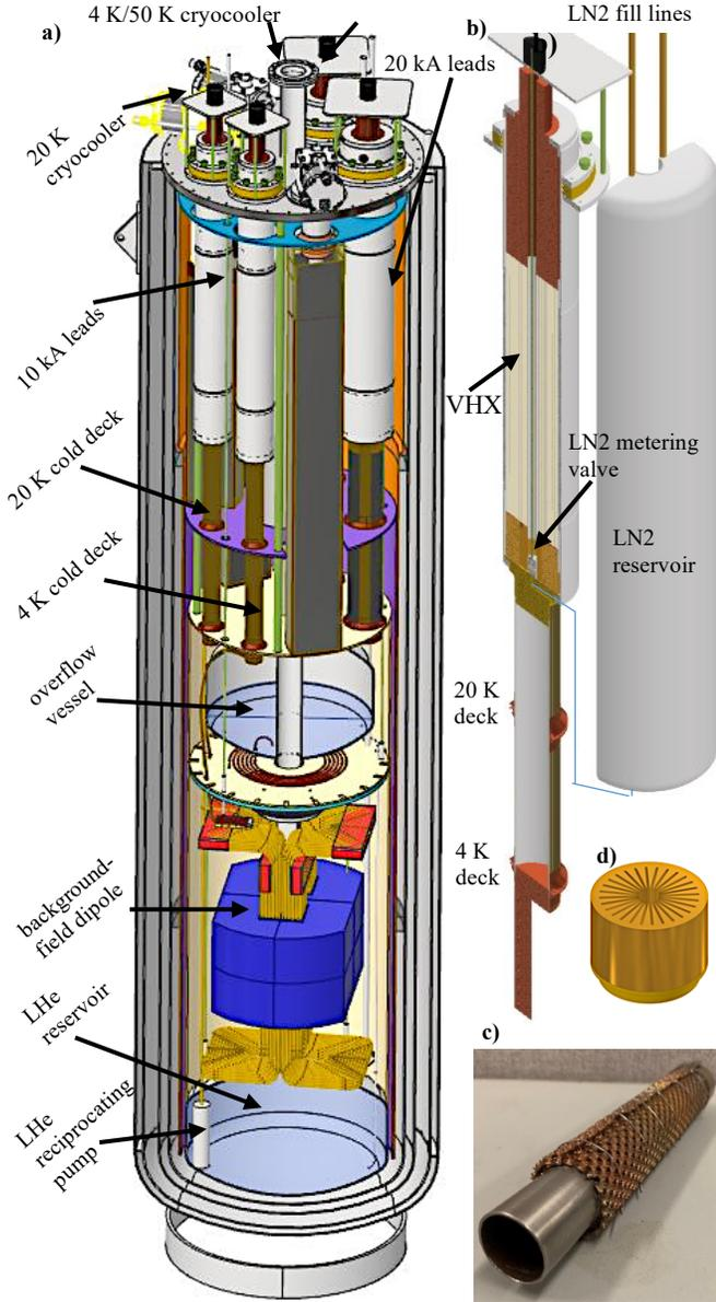
Fig. 1. Cutaway views of **a)** the test cryostat and **b)** one 20 kA ternary current lead; **c)** a sample rolling of the first two layers of the Cu jelly-roll for the VHX; **d)** detail view of the LN<sub>2</sub> manifold at the bottom of the VHX..
